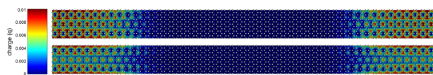
Fig. 8 Comparison of the charge distributions of the 13-AGNR-MOSFET using the WTB device Hamiltonian (above) and the produced TB device Hamiltonian (below). The gate voltage V_{GS} is set to be 0 V, and the drain-source voltage V_{DS} is set to be 0.2 V. The gray balls represent C atoms, whereas H atoms on the edges are not plotted.
