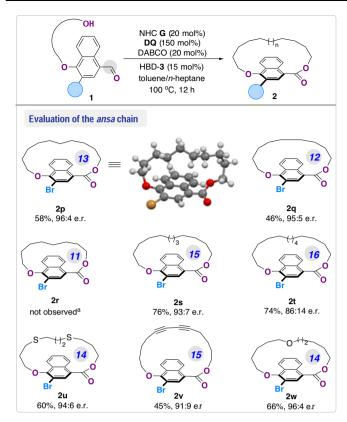
Fig. 5 | Exploration of the *ansa* chains. <sup>a</sup> The reactions were conducted with 1 (0.05 mmol, 1.0 equiv.), NHC G (5.2 mg, 20 mol%), DQ (30.6 mg, 150 mol%), HBD-3 (5.2 mg, 15 mol%), and DABCO (1.12 mg, 20 mol%) in toluene/*n*-heptane (11:9 v/v, 1 mM) under N<sub>2</sub> atmosphere at 100 °C for 12 h; Isolated yields.
