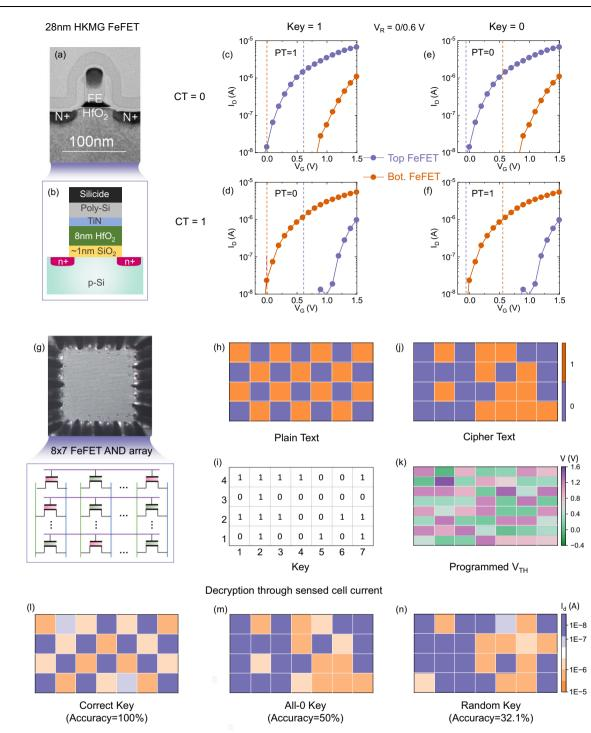
**Fig. 3** | **Experimental verification. a**, **b** TEM and schematic cross section.  $\mathbf{c} - \mathbf{f}_{I_D} - V_G$  characteristics for the proposed 2FeFET memory cell. **g** The image of 8 × 7 FeFET AND array for array-level verification.  $\mathbf{h} - \mathbf{k}$  The patterns of plaintext, keys, ciphertext, and corresponding  $V_{TH}$  after encryption.  $\mathbf{l} - \mathbf{n}$  In the decryption process, three
