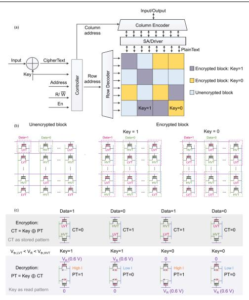
Fig. 2 | The proposed memory encryption scheme. a An overview of the proposed memory encryption architecture. b Three scenarios in the memory. c The details of the encryption and decryption schemes.
