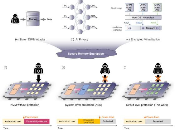
**Fig. 1** | **Motivation and potential applications.** Potential applications of memory encryption techniques: (**a**) to prevent from Stolen DIMM attacks, (**b**) to ensure AI privacy, and (**c**) to implement secure encrypted virtualization (SEV), (**d**) Without protection, NVMs become vulnerable after power down. **e** NVMs with AES-
