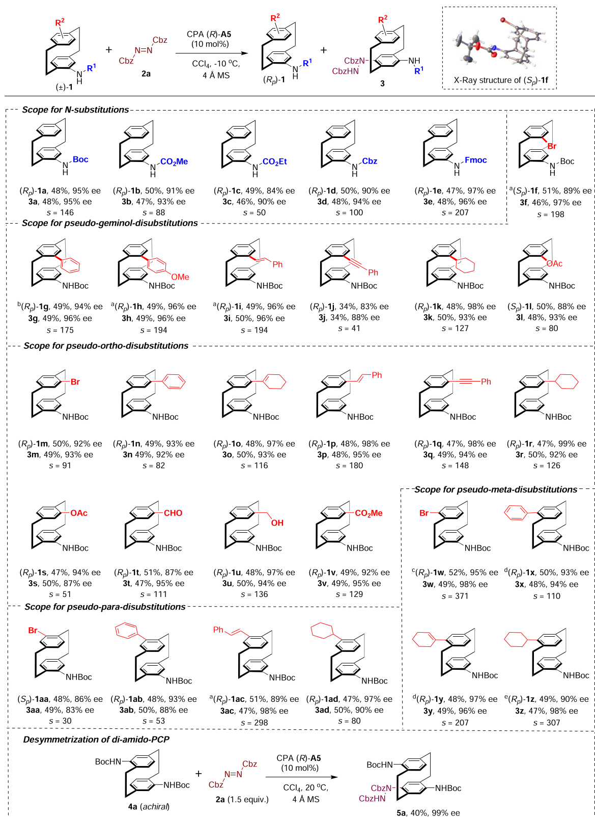
Fig. 2 | Scope for KR of substituted amido[2.2]paracyclophanes. Reactions were run with 1 (0.2 mmol), 2a (0.14 mmol) and the CPA ( R )- A5 (0.02 mmol, 10 mol%) in \text{CCl}_4 (2 ml) with 4 Å molecular sieves (200 mg) at -10^\circ\text{C} . Yields refer to isolated yields. The ee values were determined by HPLC analysis on a chiral stationary phase. Conversion ( C ) = ee_p/(ee_s + ee_p) , s = \ln[(1 - C)(1 - ee_s)]/\ln[(1 - C)(1 + ee_s)] . Note: (a)
