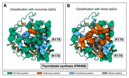
**Fig. 5** | **Analysing functional sites at a protein-protein interface.** We show the results from predicting functional sites in thymidylate synthase using either the structure of **A** the monomer or **B** the dimer as input to Rosetta for calculating  $\Delta\Delta G$ .
