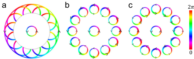
Fig. 1 | Schematics of Huygens-Fresnel principle for chiral wavelet. a–c are for continuum dielectric medium, trivial and topological photonic crystals, respectively. Color represents the phase of electromagnetic wave, and arrows indicate the transportation direction of electromagnetic energy. In b and c the thickness of circles and arrows corresponds the intensity of wavefunction and energy flow. In all cases, the wave propagation is outward, and the length scale in a should be much larger than the size of the chiral source, whereas in b and c it is the unit cell of photonic crystal. On the scale much larger than the size of unit cell, the behavior of the trivial photonic crystal can be described by a while that of the topological photonic crystal is completely different.
