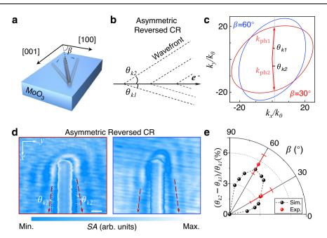
Fig. 3 | Asymmetric reversed CR in MoO<sub>3</sub>. a Schematic diagram of rotated metal nanowires on MoO<sub>3</sub> with different angles.  $\beta$  is the angle between the metal nanowire and the [1 0 0] direction of MoO<sub>3</sub>. b Schematic illustration of the MoO<sub>3</sub> phonon polaritons with asymmetric reversed CR. c Theoretical prediction of IFCs when  $\beta$  is 30° and 60°. d Experimental asymmetric reversed CR of MoO<sub>3</sub> phonon polaritons
