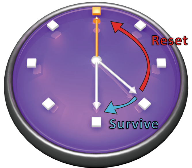
Fig. 1 | Modelling PMD processes. A PMD process with period N can be exactly modelled with N memory states. At each time step, the process either “survives” (no tick occurs) and the model advances to the next state or undergoes a tick event, and the model moves to a reset state. Due to the N -periodic nature of the conditional statistics, the model also returns to the reset state after surviving N timesteps, leading to the clock-like structure of the model dynamics as depicted.
