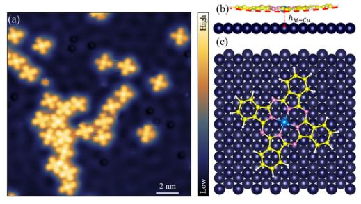
**Fig. 1** | **STM topography and schematic views of the adsorption geometry. a** Low-magnification STM image of FePc and CoPc molecules using a CO tip (*V* = 100 mV, *I* = 30 pA). Schematic side (**b**) and top (**c**) views of the relaxed FePc molecule adsorbed on a Cu(111) substrate. The red dashed curve in **b** indicates the
