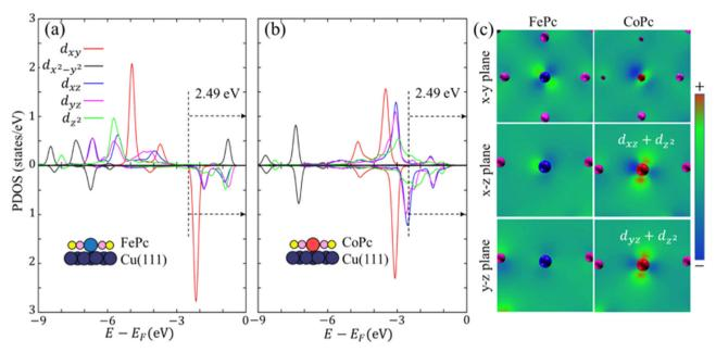
**Fig. 4** | **PDOS around the metal centers within MPcs.** DFT-computed PDOS around Fe (**a**) and Co (**b**) atoms with MPcs on Cu(111) surfaces. The top and bottom panels correspond to spin-up and spin-down states, respectively. The CO tip is excluded in these results. **c** 2D volume slice views of the combined states in an energy window of 2.49 eV below the Fermi level as indicated by the black dashed
