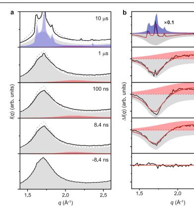
**Fig. 3** | **Structure factor before and after heating LDA. a** Experimental x-ray scattering intensities, I(q), of LDA samples measured before (gray dashed line) and after the laser excitation (black solid line). Data obtained at IR pump/x-ray probe delay times of  $\Delta t = -8.4$  ns to 10 µs are shown. Each curve is obtained from the average of I(q) over three independent x-ray shots. The contributions from LDA, HDA, and crystalline ice are indicated as gray, red, and blue shaded areas,
