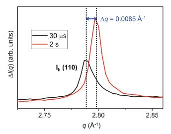
**Fig. 6** | **Bragg peak shift in ice following laser heating.** Ice  $I_h$  (110) peak positions measured at 30 µs (black) and 2 s (red) after laser excitation of the sample. The shown peak shift of 0.0085 Å<sup>-1</sup> corresponds to a temperature difference of approximately 90 K in ice  $I_h$ . As described in the text, this temperature change implies that the temperature of the LDA sample was increased by 60 K by the IR laser pulse, prior to crystallizing.
