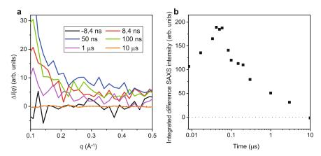
Fig. 5 | Small-angle x-ray scattering results. a The difference between the unpumped and pumped scattering curves at various time delays in the SAXS region. b Timedependent integrated difference SAXS intensity from q = 0.1 to 0.3 Å<sup>-1</sup>.
