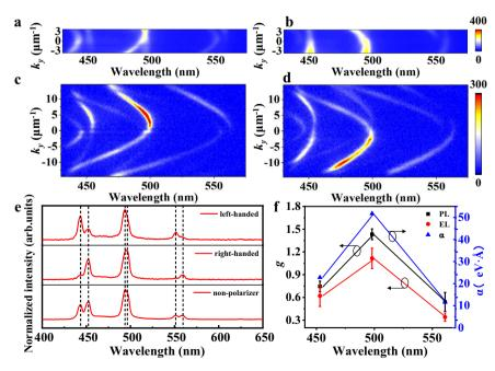
**Fig. 4** | **Angle-resolved EL measurements.** Polarized angle-resolved spectra of EL (**a**, **b**) and PL (**c**, **d**). The units of the color bars are arbitrary. **e** EL emission spectra of unpolarized,  $\sigma$ + and  $\sigma$ - components. **f** Wavelength-dependent spin-splitting
