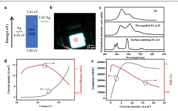
**Fig. 3** | **EL architecture and performances. a** Energy level diagram of the device. **b** Photomicrograph of the 6M-DSB single-crystal OLED array under EL. **c** Upper: PL spectrum of the 6M-DSB crystal. Middle: spectrum of the crystal edge waveguide under EL as shown in **b**. Lower: spectrum of light emanating from the microcavity
