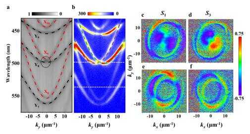
**Fig. 2** | **Reflection and PL measurements. a** ARR and **b** ARPL of the microcavity with the organic-layer thickness of 990 nm. The units of the color bars are arbitrary. The dotted curves in **a** represent the simulated X and Y cavity modes, respectively. The dashed curves in **b**, indicating the split CP modes, are calculated by solving Eq. (1) with the parameters  $E_0 = 2.495$  eV (497 nm),  $m = 2.2 \times 10^{-5} m_e$  ( $m_e$  is the free
