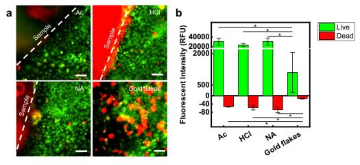
**Fig. 6 Biocompatibility of UCDEs. a** Confocal imaging of live/dead stained HaCaT cell cultured for 7 days (scale bar,  $100 \mu$ m). The sample group of a soaking method for UCDEs: Acetone (Ac), Hydrochloric acid (HCl), Nitric acid (NA), and gold flakes. **b** Relative fluorescence intensity of cells cultured for 7 days is presented as average and standard error of means (\*p < 0.05 TTEST).
