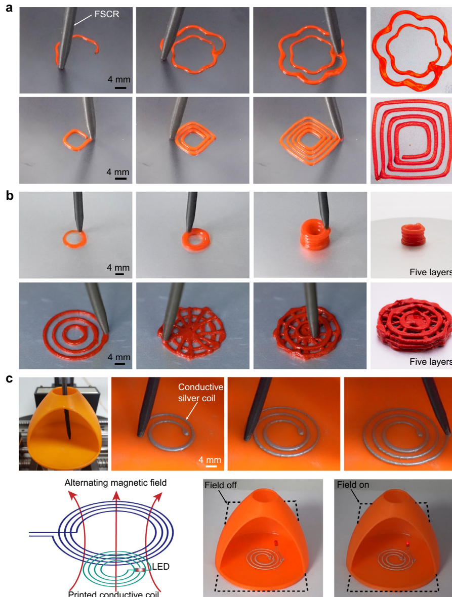
Fig. 4 Direct ink printing by an FSCR. a Demonstration of FSCR printing with viscoelastic materials (PDMS-1700 and Ecoflex composite) into different patterns such as a flower with six petals and a square spiral. b Printing 3D five-layered tube and scaffold with viscoelastic materials. c Upper panels: Images of experimental demonstration of printing functional device. An LED was placed as an energy-dissipating element on a conductive silver ink coil after printing. Bottom panels: left, schematic of the printed wireless device that powered a surface-mounted LED under an alternating magnetic field from an electromagnetic coil (power: 1600 watts) at a distance of 10 mm. Middle: the actual circuit. Right: LED activation upon imposing an alternating magnetic field.
