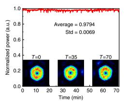
**Fig. 7 Long-term stability.** The normalized power of the correlation signal collected by the SMF, indicating stable phase locking over 70 min. The inserts are examples of beam intensity profiles measured at different times, showing that the doughnut-shaped beam was well preserved during the measurement period.
