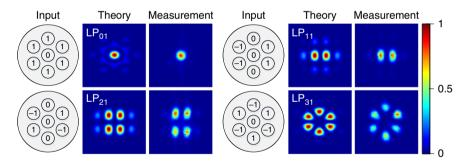
Fig. 4 Scalar LP mode generation. Idealised complex amplitudes of the individual cores required to generate specific LP fibre modes and the corresponding beam profiles in the far-field (in theory and measurement).
