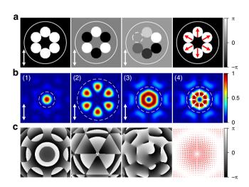
**Fig. 1 Calculation of coherently combined modes from a 6-core MCF. a** Examples of phase and polarization distributions of the MCF beamlets for the generation of various structured light beams. **b**, **c** Calculated far-field (**b**) intensity, (**c**) phase or polarization state distributions of the synthesized modes (white and red arrows show the polarization orientations).
