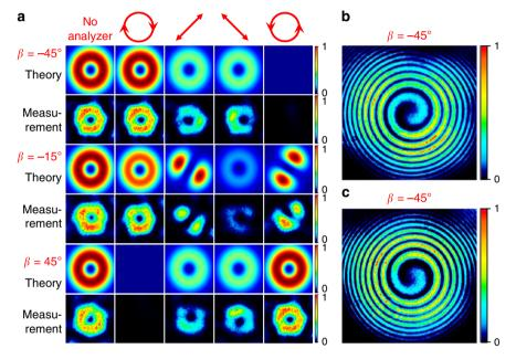
**Fig. 6 OAM beams. a** Theoretical (odd rows) and experimentally measured (even rows) output beams and the corresponding intensity profiles after passing through a rotated circular polarizer in the case of  $\beta = \pm 45^{\circ}$  and  $\beta = -15^{\circ}$ . **b** The measured spiral interference fringes of the generated vortex beams with opposite handedness when  $\beta = \pm 45^{\circ}$ .
