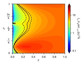
**Fig. 2** Thermally averaged loss rate coefficient from the single-channel model at 1.5  $\mu$ K.  $k_2(T)$  is plotted as a function of the loss parameter y and the short-range phase shift  $\delta^s$ . The solid and dashed black lines correspond to the measured  $k_2$  and uncertainty, respectively
