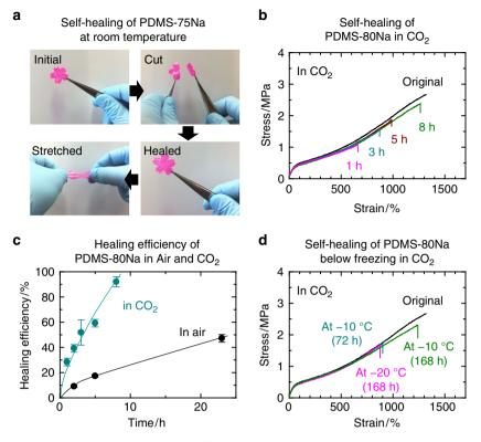
**Fig. 4** Effect of  $CO_2$  on self-healing of PDMS-xNa. **a** Photograph of self-healing behavior of cherry blossom-shaped PDMS-75Na film at 26 °C. The film was painted pink. **b** Stress-strain curves of PDMS-80Na healed at 26 °C in  $CO_2$ . **c** Time variation of healing efficiency of PDMS-80Na stored at 26 °C in air and in  $CO_2$ . The error bars indicate standard deviations. **d** Stress-strain curves of PDMS-80Na healed at -10 °C and -20 °C in  $CO_2$ .
