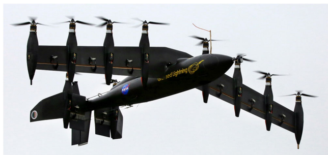
Fig. 2 NASA GL-10 VTOL 1 . The takeoff and landing hover configuration for a prototype NASA VTOL is shown here. The tilt rotor and wing design combines the convenience of local takeoff and landing like a helicopter with the efficient aerodynamic flight of an airplane
