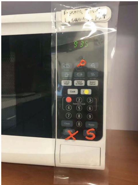
Fig. 4 Example of tactile marking on microwave. Tactile markings, in this example, allow for recognition of critical buttons allowing the microwave to be used.
