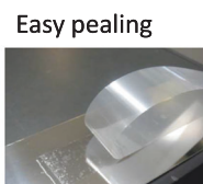
Fig. 8 a Thermal degradation of the polyperoxide synthesized from diene monomers. For PPMS, the ester alkyl group R is methyl. b Result of a 180° peeling test for PPMS at room temperature before heating. The T_g of PPMS is -13^\circ\text{C} , which is higher than the ideal T_g value for PSA. As a result, a stick–slip phenomenon is observed. c Result of a 180° peeling test for PPMS at room temperature after heating at 70^\circ\text{C} for 1 h. The peel strength is drastically reduced, and the adhesive tape is easily released from the a stainless-steel (SUS) plate as the adherend. The peeling test is carried out at room temperature
