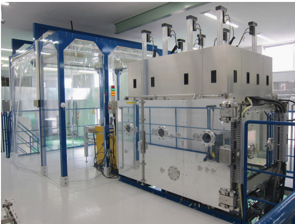
Fig. 4 Pilot plant for plasma chemical vapor deposition (CVD)
