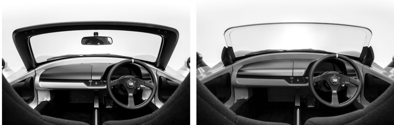
Fig. 10 Conventional glass front window with an A-pillar (left) and a newly developed pillar-less front window (right)
