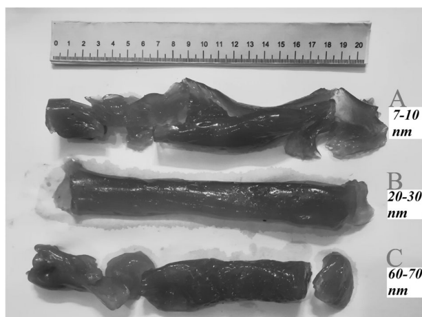
Fig. 12 The difference between gel columns for gel number 4, 8 and 12 after reaching their maximum DCP. The gel column length and diameter for these cases was 200 and 25.4 mm, respectively
