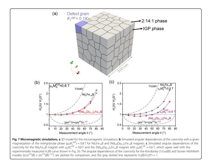
the pinning strength of the intergranular phase against the demagnetization process of samples was additional evidence for the different magnetic hardening mechanisms, which agreed with the results on the angular dependence of the coercivity shown in Fig. 2b.
