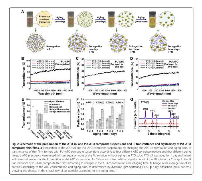
with different ATO concentrations aged for different durations were mixed with the same amount (5 g) of a 16.7 wt% PU solution in the DMF-THF cosolvent (3:2 ratio), and stirred evenly for at least 6 h to prepare the PU–ATO composite suspensions. To verify the optical properties of the prepared PU–ATO composite suspensions with different compositions, their transmittance in the NIR range was evaluated by ultraviolet–visible–near-infrared (UV–vis–NIR) spectroscopy.
