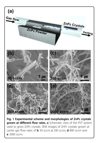
ZnPc vapors to a cooler region. A silicon substrate was placed at the end region of the furnace where the temperature naturally decreased to collect resulting crystals efficiently (Fig. 1a). After 10 min of reaction, blue ZnPc crystals were formed at the end of the tube furnace.
