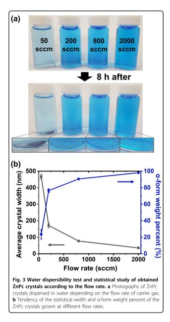
without significant precipitation. These results agree well with the PXRD data that show an increased ratio of  $\alpha$ -form ZnPc as the flow rate of the carrier gas increased.
