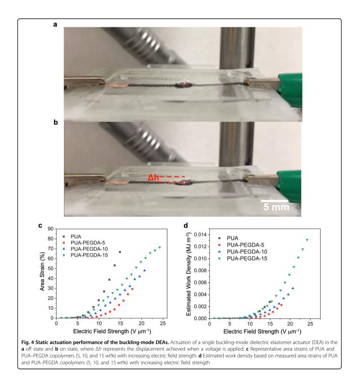
observed in the PUA–PEGDA copolymers (PUA–PEGDA-X, where X is the wt% of the PEGDA). This finding is attributed to the nonlinear behavior of PUA, for which the modulus becomes significantly smaller than that of the PUA–PEDGA copolymers (Fig. 3a) beyond 10% strain. The early breakdown of PUA is expected without the application of prestrains to prevent electromechanical instabilities. In contrast, copolymers
