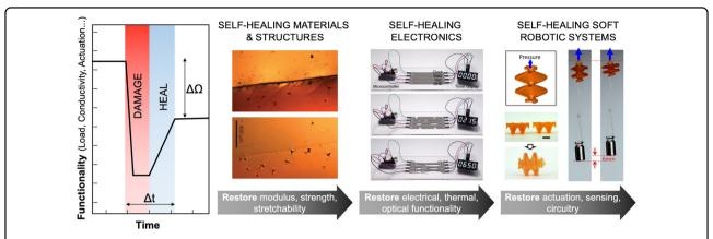
**Fig. 1 Modes of self-healing in soft material systems.** The self-healing response of a material can be characterized by the damage response time ( $\Delta t$ ) and recoverability/loss ( $\Delta \Omega$ ) of material functionality. Such functionality can relate to structural load bearing <sup>13</sup>, electrical conductivity<sup>8</sup>, or robotic actuation<sup>23</sup>
