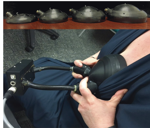
Fig. 1 OBS cups and device. Photo demonstrating the four OBS measurement cup sizes in the top photo and the OBS device in use on a participant in the bottom photo.
