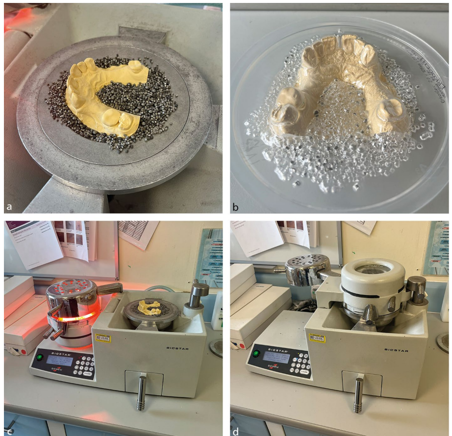
Fig. 3 a) The casts are embedded in stainless steel granules to avoid stretching of the material during push down which would stretch the material and result in occlusal thinning. b) Untrimmed, maxillary splint. c) Thermosoftening material being pre-heated to its working temperature. d) The softened disk cooling off after being pushed down onto the maxillary cast
