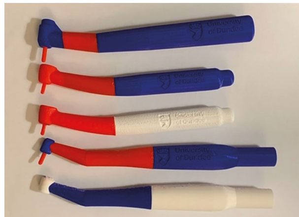
Fig. 2 Varying prototypes investigating the balance of conductive and non-conductive materials
