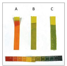
Fig. 1 pH testing strip results. A – Surgicel in normal saline: B – Normal saline: C – Alveogyl in normal saline
