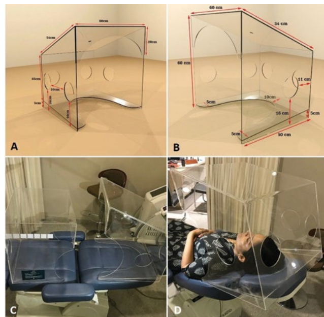
Fig. 1 Modified aerosol box design for viable dentistry
