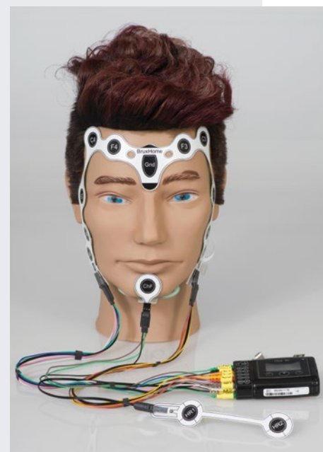
New polysomnography electrode set enables easy at-home assessment of sleep bruxism
