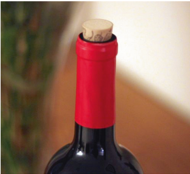
Fig. 4 Cork protrusion after exposure to excessive heat
