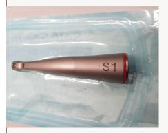
ES Precision has helped an Oxfordshire dental practice to keep track of dental tools without the need for label application or hard-to-read serial numbers. The laser marks are permanent, clear and withstand repeated autoclaving.
