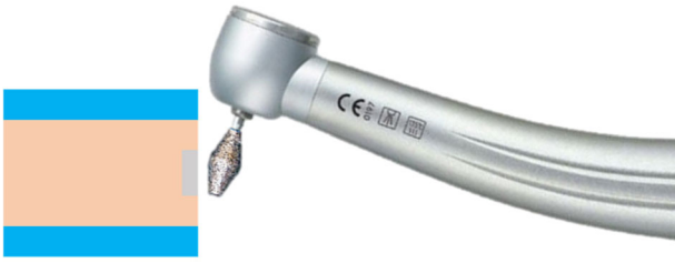
Fig. 2 Bur grinding of the zirconia specimen. A double cone-shaped diamond bur aligned with a flat surface parallel to the specimen surface was attached to a high-speed airtor, which was connected to the computer numerical control.
