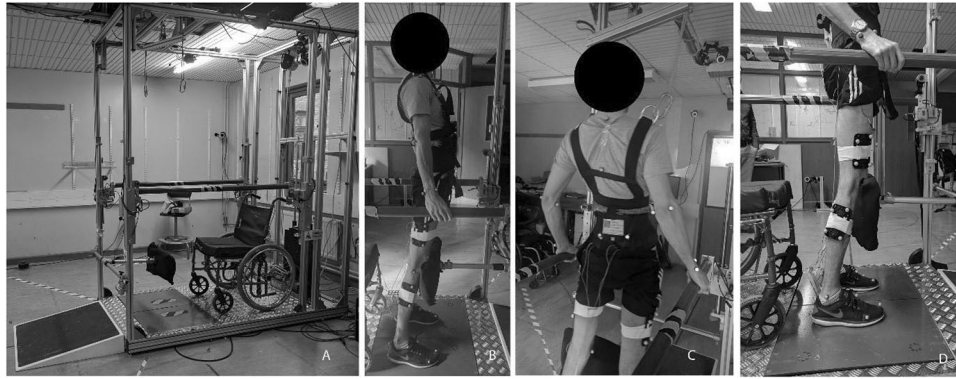
Fig. 1 FES assistive standing Frame. A Novel standing system for load shifting exercises, B–D Participant standing for FES-assisted weight shifted exercises and infrared markers.
