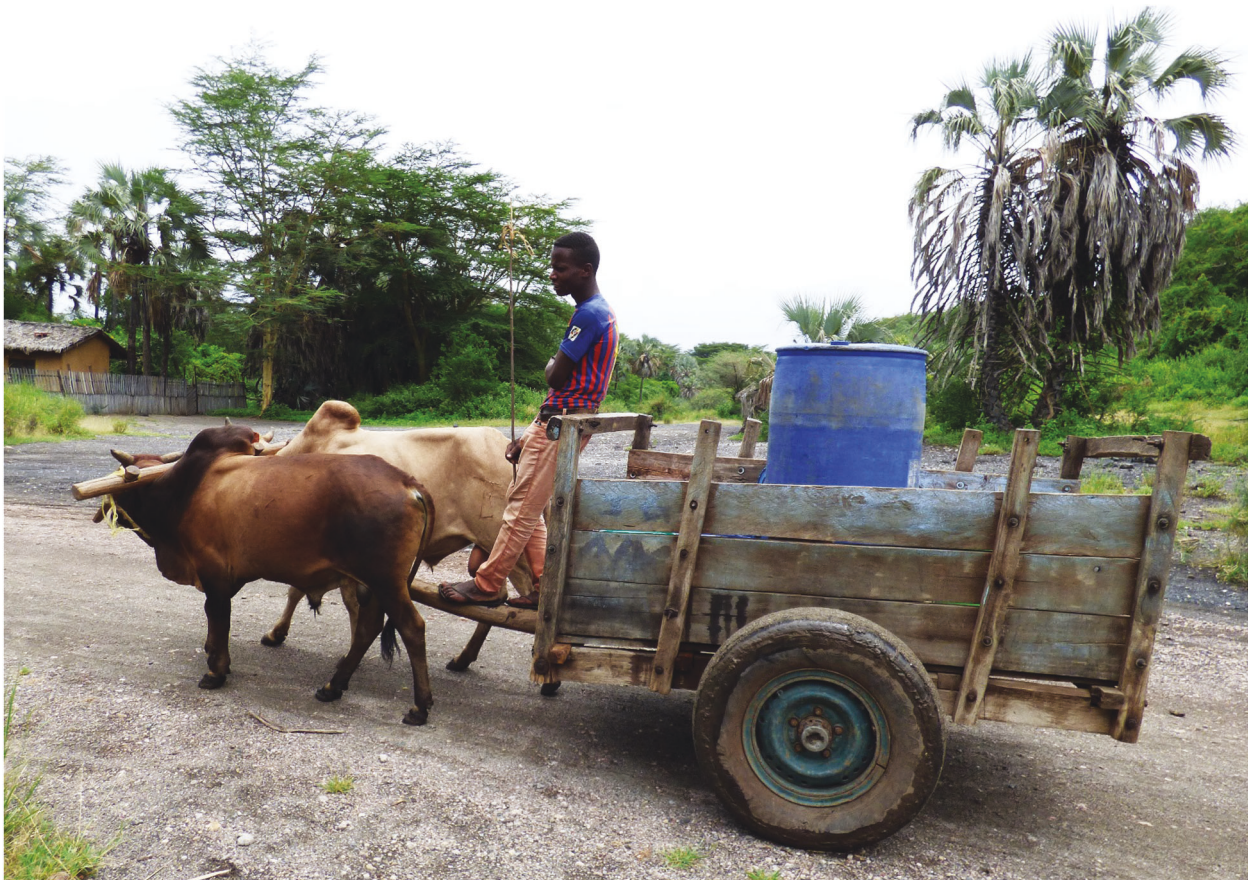
Fig. 1 An ox-cart with a water-filled container and the rider. The ox cart is mainly made of wood, with less safety considerations and their riders hardly take any precautions.
