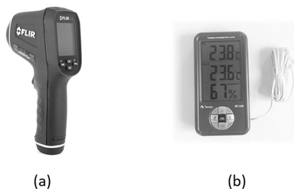
Fig. 1 Devices for the Tsk Measurements. a Noncontact infrared thermometer FLIR TG 165, and b MT-240 hygrometer/thermometer.
