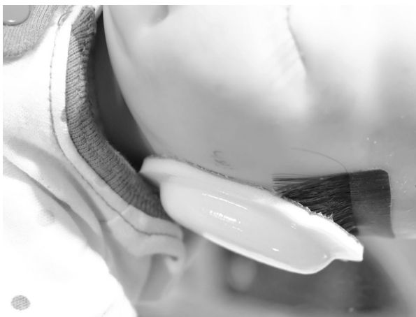
Fig. 2 Ear covers adhered to manikin with hair extensions. Test conditions included ear covers adhered to the manikin over the auricles and adhered to the manikin over hair extensions that simulate the hair present in many infants.
