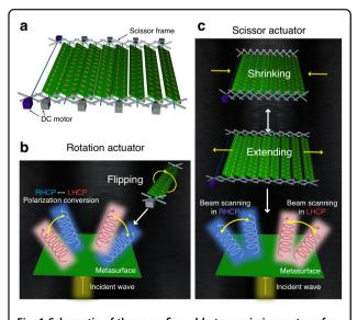
**Fig. 1 Schematic of the reconfigurable transmissive metasurface with a combination of scissor and rotation actuators for independent control of beam scanning and polarization conversion. a** The metasurface model. **b** Unit cell rotation controlled for the polarization conversion function. **c** Space controlled by blue DC motors for beam scanning functions
