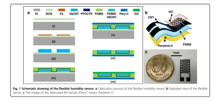
an E-beam evaporator and patterned for an interdigital finger shape with a lift-off process (Fig. 1a(ii)). Then, the VACNT forest (Fig. 1a(iii)) was synthesized using the microwave plasma-enhanced chemical vapor deposition (PECVD) apparatus to form the sensor electrodes.
