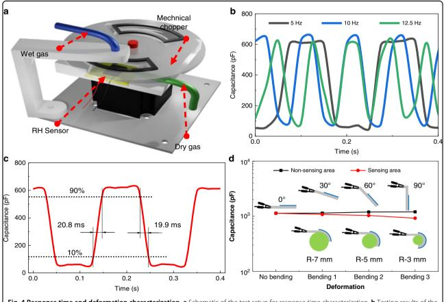
**Fig. 4 Response time and deformation characterization. a** Schematic of the test setup for response time characterization. **b** Testing results of the capacitance change of the flexible humidity sensor under different switching frequencies of the mechanical chopper. **c** Response and recovery characterization. **d** Deformation test of the flexible sensor under bending nonsensing areas and sensing areas
