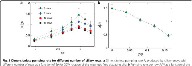
Fig. 5 Dimensionless pumping rate for different number of ciliary rows. a Dimensionless pumping rate  $P_f$  produced by ciliary arrays with different number of rows as a function of *Sp* for CCW rotation of the magnetic field actuating cilia. **b** Pumping rate per row  $P_f/N$  as a function of the normalized distance *C/D* of the magnet from the center for an array with N = 3. The arrays have 25 cilia per row with spacing  $S = 300 \,\mu\text{m}$ . Channel height is  $H = 300 \,\mu\text{m}$
