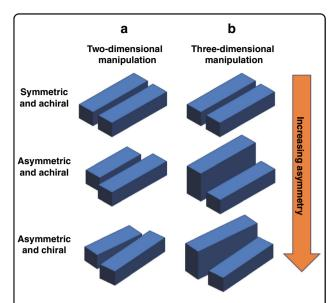
**Fig. 1 BIC to qBIC by breaking the symmetry of resonator geometry. a** Two-dimensional and **b** three-dimensional geometric manipulations of anti-parallel rods that can make up the unit cell of a qBIC metasurface. (Top) Symmetric, achiral rods. (Middle) Through resonator symmetry-breaking, the rods comprise an asymmetric unit cell. (Bottom) By tilting the rods towards one another, the unit cell becomes chiral
