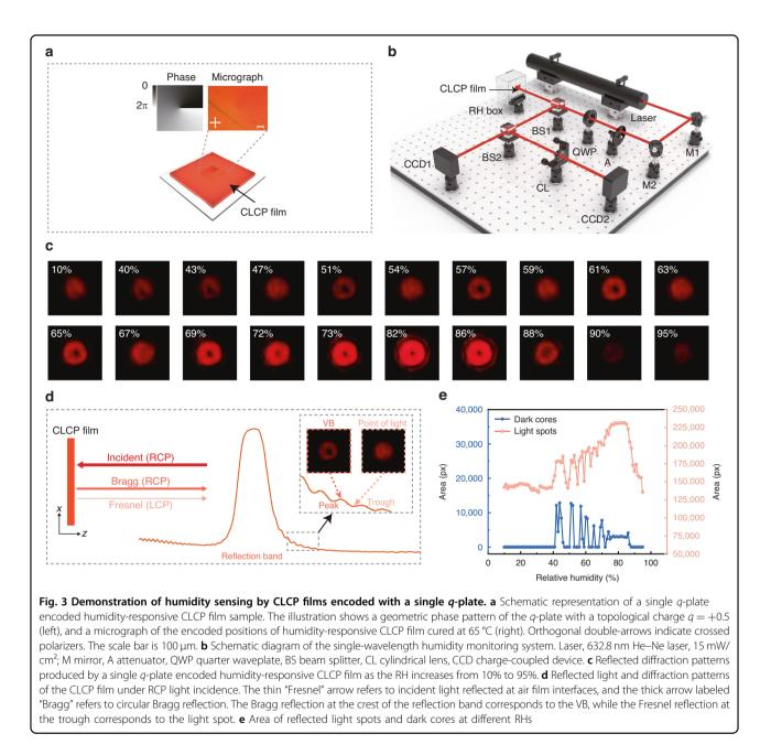
a wavelength shift of the reflection maximum ranging from 581 to 719 nm, corresponding to a variation of RH between 10% and 95%.
