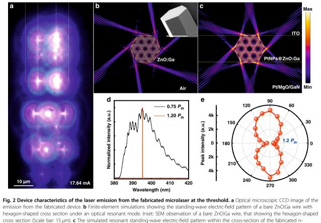
PtNPs@ZnO:Ga MW/Pt/MgO/p-GaN emission device structure. **d** Normalized EL emission spectra of the fabricated device for two injection currents below (0.75  $P_{th}$ ), and above (1.20  $P_{th}$ ) the laser threshold, respectively. **e** Polarization properties of the laser emission for an operating current above the threshold (~1.20  $P_{th}$ ). The experiment EL data are symbolized by the red dots and the red solid line is the fitting result
