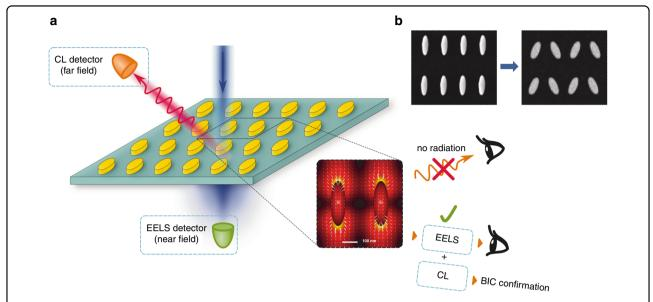
Fig. 1 Schematic for exciting and probing bound-states-in-the-continuum (BIC) modes. a Experimental STEM setup is used to focus a high-energy electron beam to probe a dielectric metasurface. Complementary measurements of the energy lost by electrons, and energy of emitted photons result in EELS and CL spectra respectively. b Transformation of BIC into quasi-BIC
