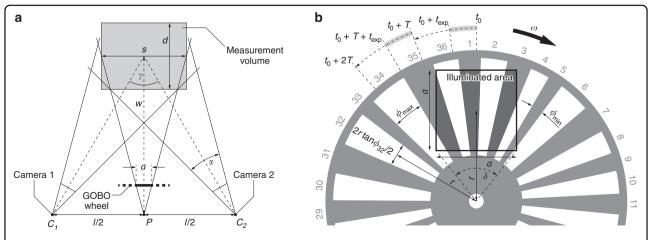
**Fig. 1 Schematic illustration of a GOBO projection-based 3D sensor.** Definitions of some of the variables that are listed in Table 1 by means of **a** a top view of the camera-projector-camera arrangement and **b** an exemplary GOBO wheel with aperiodic binary fringes
