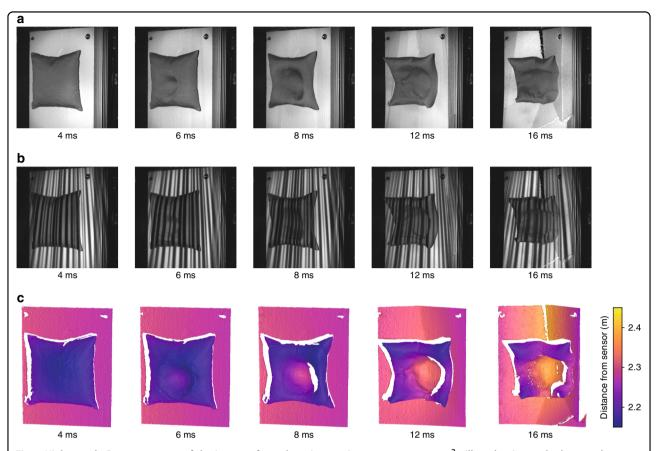
Fig. 4 High-speed 3D measurement of the impact of a 40-bar nitrogen jet on a 400 × 400 mm<sup>2</sup> pillow that is attached to a polystyrene plate. a Snapshots of the recorded process at five points in time. b Camera images of the GOBO-projected aperiodic sinusoidal fringes, which are recorded with a resolution of 512 × 408 px at a frame rate of 55.2 kHz. c Reconstructed point clouds at a 3D rate of 5.5 kHz (see also Supplementary Video S2)
