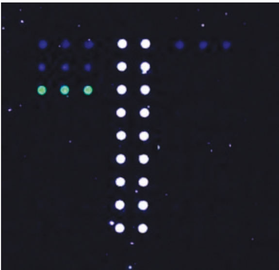
Figure 2. The result of microarray hybridization of S. aureus showed in Fig. 2. Visible spots are located in line 1 (Universal probe 1), line two (Universal 2), line three (Gram-positive) and line five ( S. aureus ),
