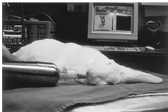
Figure 1. Experimental setup showing the delivery of labeled salbutamol pressurized metered-dose inhaler (Ventoline) from a small-volume spacer device in lightly anesthetized and intubated (Portex 3.0-mm endotracheal tube) spontaneously breathing New Zealand White male rabbits.
