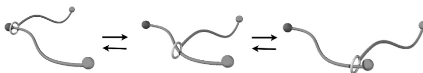
Figure 1 Transformable polymer based on a rotaxane structure. A full color version of this figure is available at Polymer Journal online.
